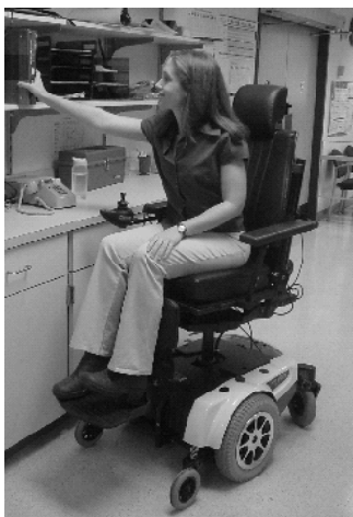
Figure 10. Example of an electric powered wheelchair with powered seat elevation function.
