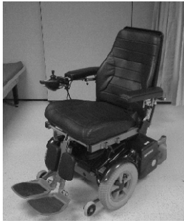
Figure 6. Example of a front wheel drive electric powered wheelchair.
