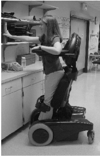
Figure 11. Example of an electric powered stand-up wheelchair.
