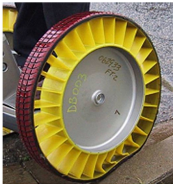
Figure 5: Early Tweel™ assembly prototype
