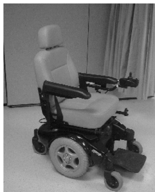
Figure 5. Example of a mid-wheel drive electric powered wheelchair.
