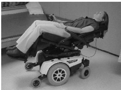
Figure 8. Picture of an electric powered wheelchair with a power seat recline.
