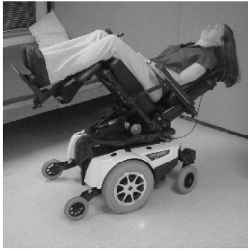
Figure 9. Picture of an electric powered wheelchair with power seat tilt function.
