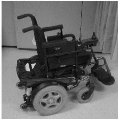
Figure 4. Picture of a rear-wheel drive electric powered wheelchair.
