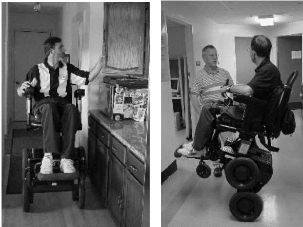
Figure 13. An IBOT in balance function.
